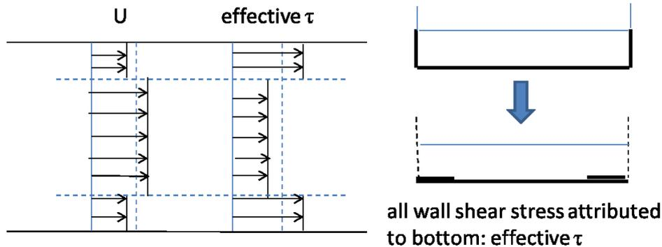
Figure 5. Analogy of influences of side wall shear stresses and thixotropy (adverse relation between variation of flow velocity and variation of bed shear stress)
